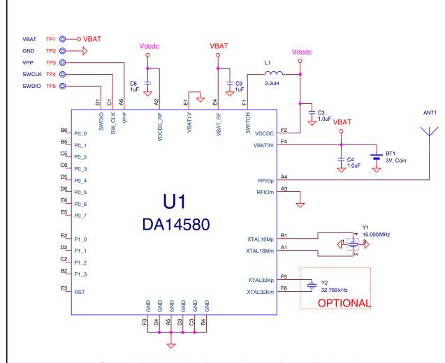
Figure 12 Lithium coin cell powered system diagram (Buck mode)
