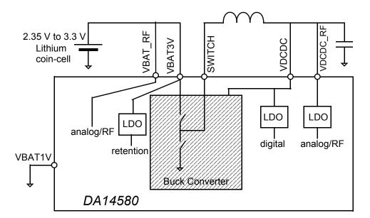
Figure 8 Supply overview, Coin-cell application
