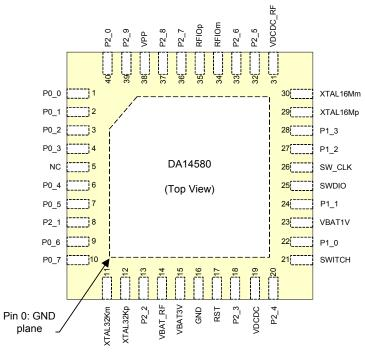
Figure 4 QFN40 pin assignment
