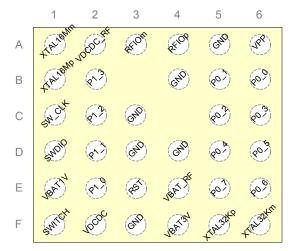
Figure 2 WLCSP34 ball assignment
