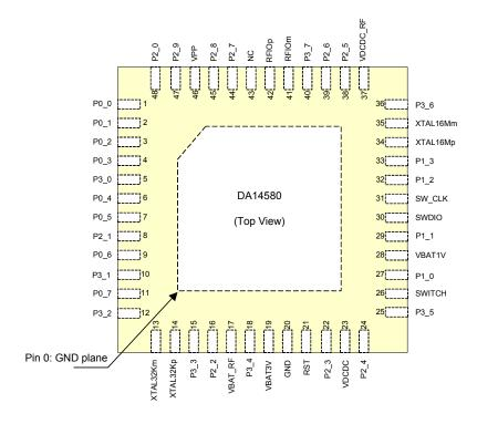
Figure 3 QFN48 pin assignment
