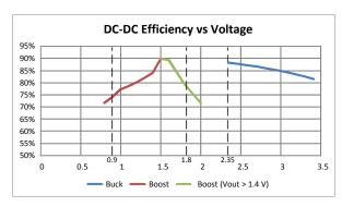
Figure 10 DC-DC efficiency in Buck/Boost mode at various voltage levels
