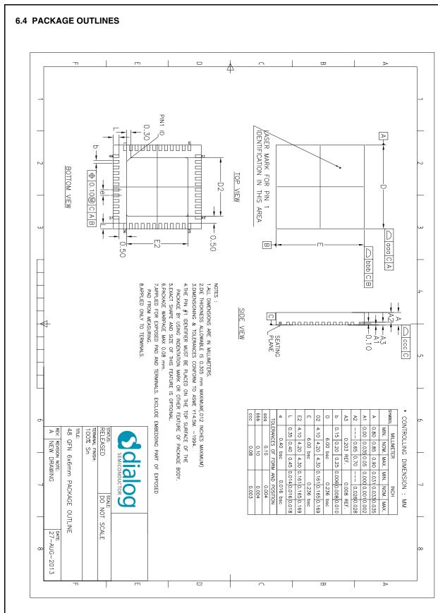
Figure 13 QFN48 Package Outline Drawing
