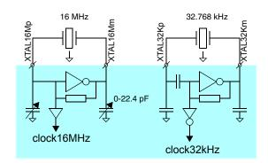
Figure 7 Crystal oscillator circuits
