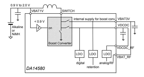
Figure 9 Supply overview, Alkaline-cell application
